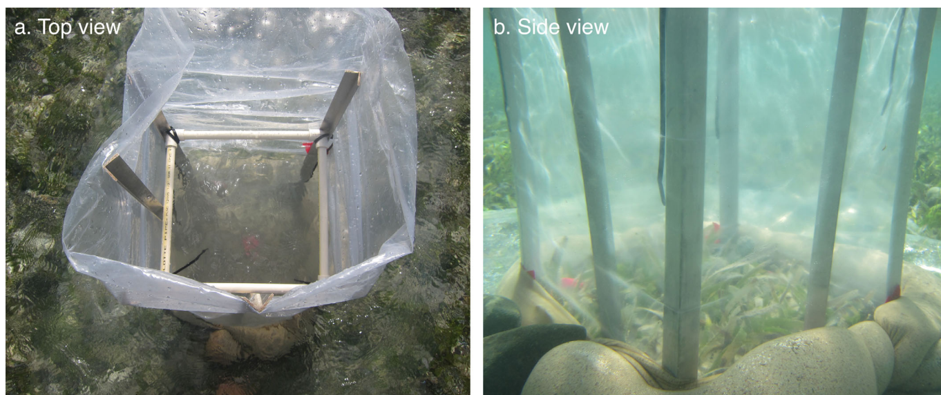
Fig. 2. Photos show the enclosures from above (a) where they were left open so air–sea gas exchange could occur, and how water residence times were increased by enclosing the plots with plastic lining weighed down with sand bags (b).
