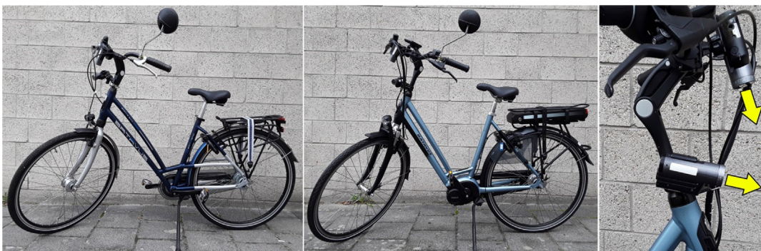
Fig. 2. The regular bicycle (left), the pedelec (centre), and the position of the GPS action cameras (right).
