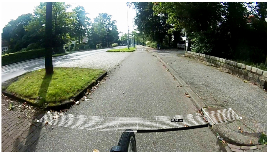
Fig. 4. Lateral position measurement by overlaying a perspective grid (white) on the video using Kinovea. The perspective grid represented the absolute dimensions (300 × 30 cm) in front of the bicycle's front wheel.
