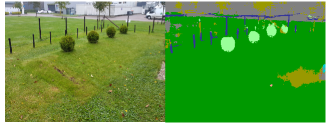
Figure 6 A view of the Wageningen test garden (left) and the output of the semantic segmentation algorithm (right).
