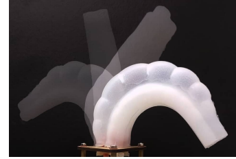
Figure 1: Elephant-inspired soft robot manipulator made from flexible material. Video: https://goo.gl/bJJJvu
