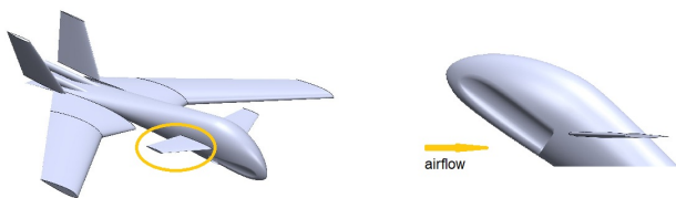
Figure 1: (left) Conceptual design of the FSW UAV. The canard is indicated in orange. (right) Neutral canard angle
