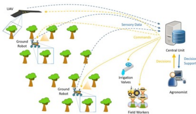
Figure 1: Idea of the SCADA system for agriculture.
