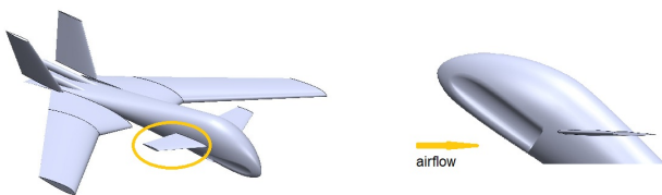
Figure 1: (left) Conceptual design of the FSW UAV. The canard is indicated in orange. (right) Neutral canard angle
