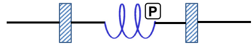
FIG. 3. A generalized barrier-CISS center-barrier (BCB) model for P -type CISS molecules. The ideal, 100%-spin-selective CISS center in the middle introduces the directional spin transmission in a CISS molecule, while the two identical nonmagnetic barriers (with transmission probability t ) contribute the nonideal electron transmission and reflection behavior. The overall transmission and reflection matrices of the entire BCB module are fully determined by t and have all elements taking finite values between 0 and 1.
