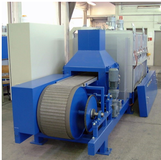
Figure 2.6. Industrial sized pushbelt furnace (at Philips Drachten).
