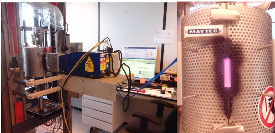
Figure 2.7. Tensile bench equipped with a furnace and a laser extensometer installed in front of the furnace.
