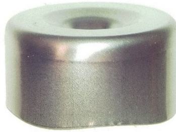
Figure 2.1. Cup made by deep drawing of a round blank. Earing is seen on the open side of the cup, facing the bottom of the image.
