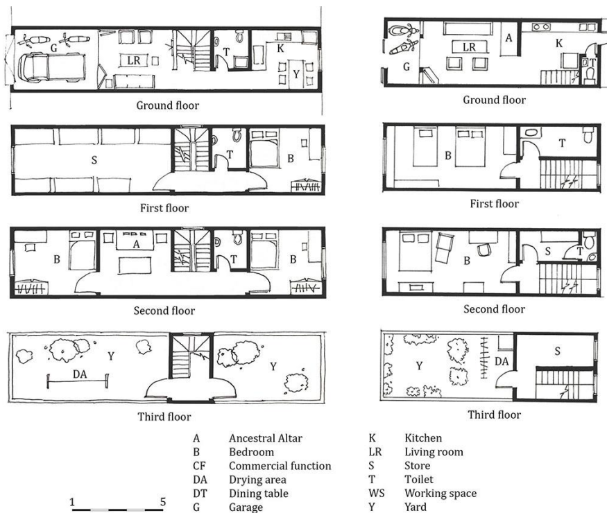
Figure 6: Examples of contemporary self-built house plans after the economic reform (Drawn by Ngo Kien Thinh)
