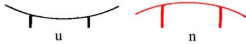
Figure 2. Schematic representation of both sample position. In the “u” concave position, the radius is underestimated due to the gravity that pulls at the specimen. The radius is overestimated for the “n” convex position.
