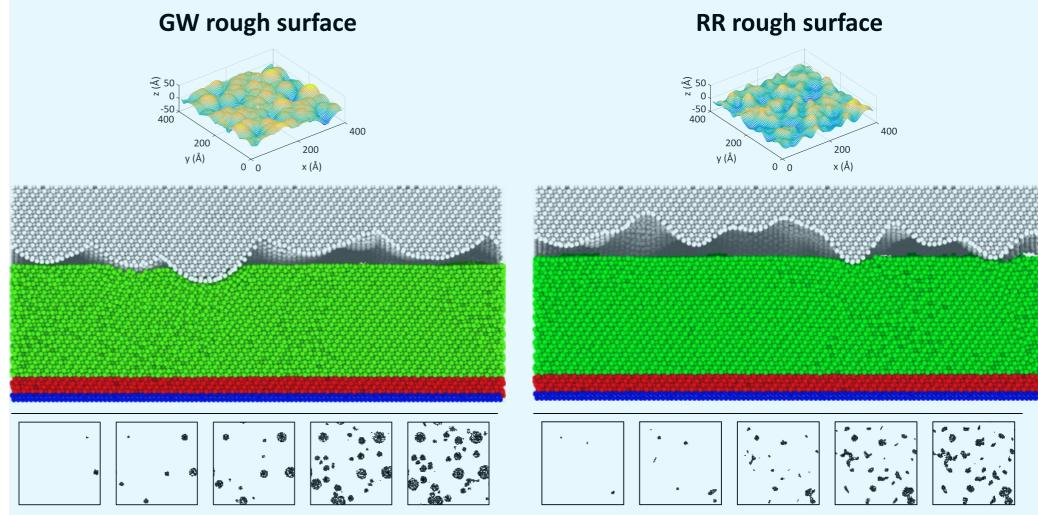
**Contact Evolution:** The black dots indicate the contacted atoms of the rough surface contacts at different nominal pressure values.
