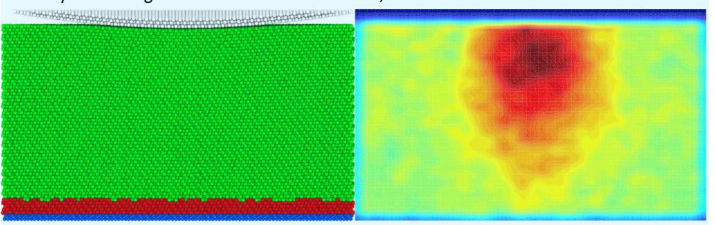
**Contacting system: (Left)** A spherical cap indenter of R=1000~Å indents an atomically flat substrate. The blue, red, green, and white dots represent the fixed, thermostatic, Newtonian, and indenter atoms. (**Right**) The system's responses were collected up to the point before which the stress fields were affected by the boundaries.
