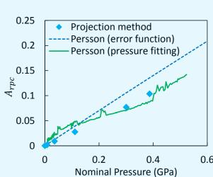
The values of  $A_{rcp}$  for both systems showed the same dependence on normalized pressure. Moreover, the results show that the studied rough surface contact theories underestimate the contact areas; however, the Persson theory resulted in closer estimations for  $A_{rcp}$  calculated based on fitting the interfacial pressure distribution.
