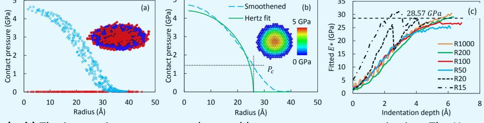
(a, b) The interacting atoms were detected by a non-zero pressure criterion. The Hertz formula was fitted to the smoothened data, only after the background noise was removed with a threshold of  $0.02\ GPa$ .
