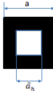
Figure 3.6: Mesostructure unit for density calculation
