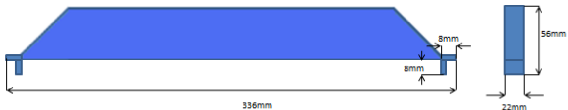
Figure 5.15: Dimensions of the MBB beam – SIMP and HOMOG-B
