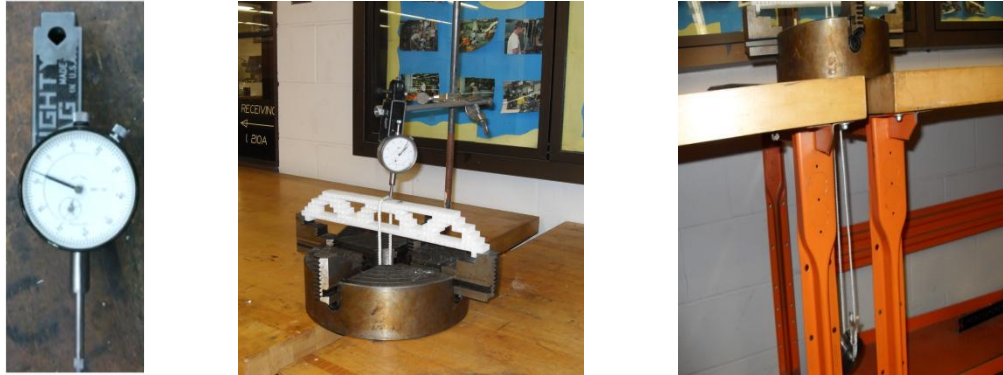
Figure 5.12 Test set up equipment – Dial Indicator, MBB SIMP case and weights
