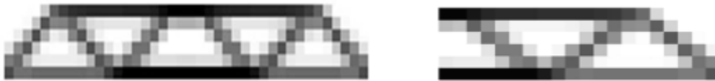
Figure 4.7: SIMP solution for the MBB beam problem – Full beam and half beam
