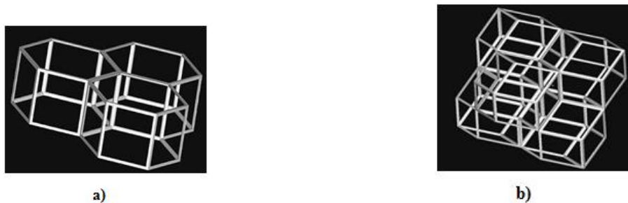
Figure 1.3 Cell structures studied by Cheah a) three hexagonal prisms b) five rhombic decahedrons
