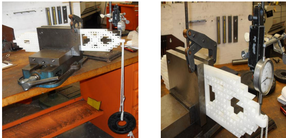
Figure 5.14: Cantilever beam test set up – Dial Indicator, Vise blocks, weights and clamp at the top
