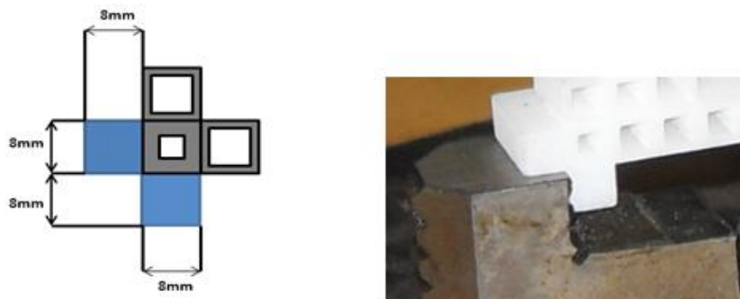
Figure 5.11: Mount designs for the MBB beam
