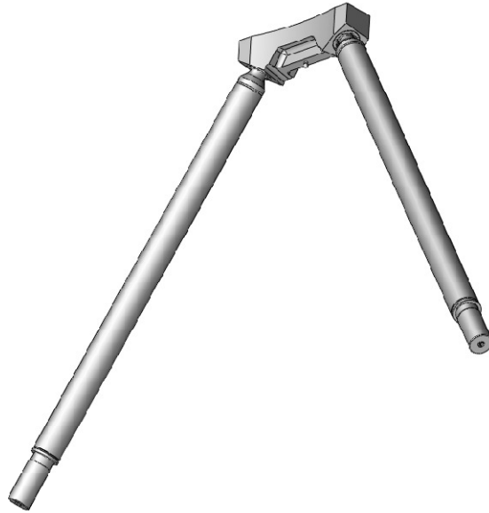
Figure 6-6: The completed upper bi-pod assembly is shown [24].
