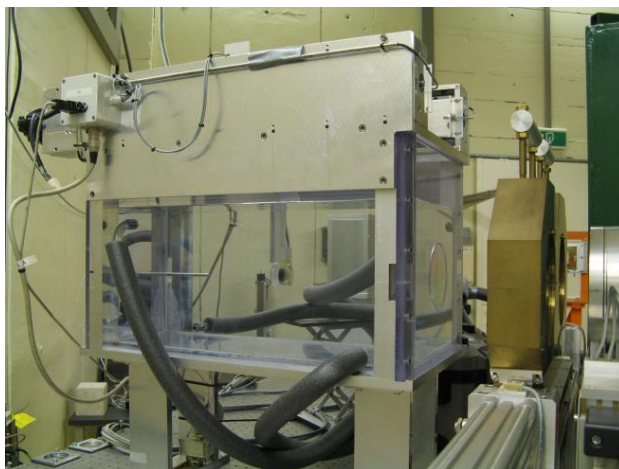
Figure 4.1. Experimental setup of the water phantom with its entrance window placed at the device under test (DUT) position. An ionization chamber is positioned in the water phantom on a translation stage to enable measurement of depth dose profiles.
