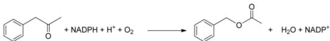
Figure 3. Schematic representation of the reaction catalyzed by phenylacetone monooxygenase (PAMO): a Baeyer-Villiger oxidation of phenylacetone into benzyl acetate.
