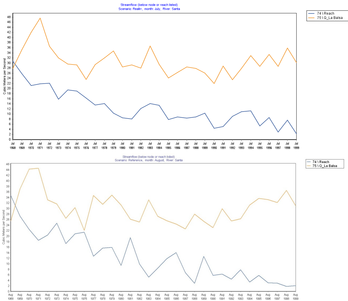
Figure 27: Monthly stream flow for July (top) and August (bottom) at La Balsa from 1968-1999, comparing the model (blue) to the observed gauge flow (orange)
