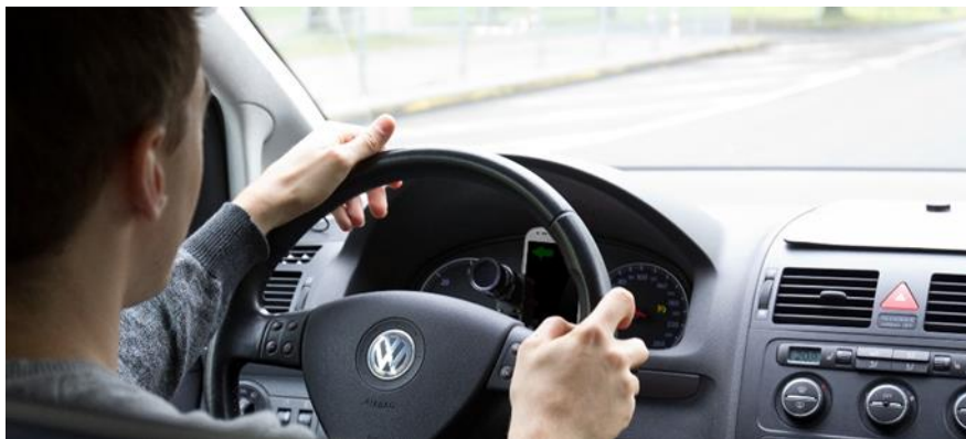
Figure 1. Driver camera and smartphone application for automated indicator function in the test vehicle
