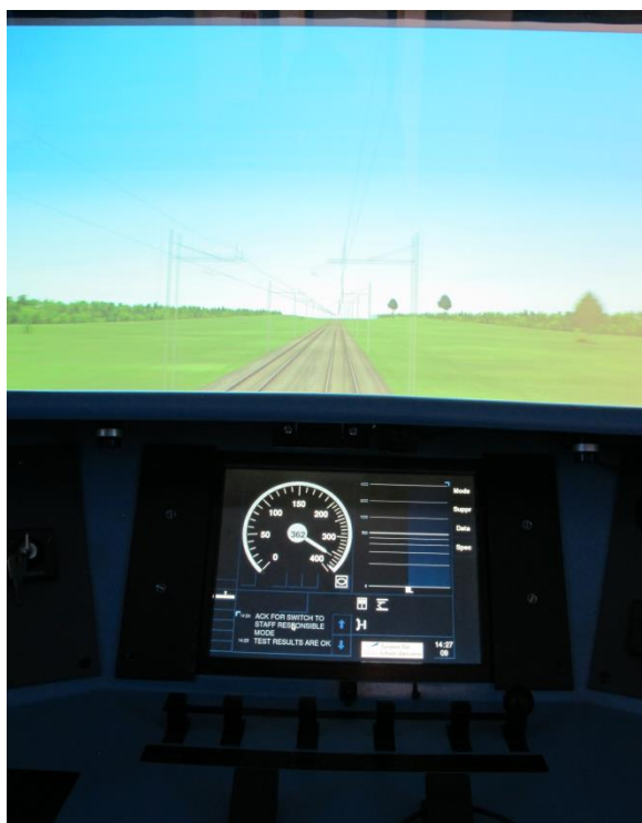
Figure 2. High fidelity railway simulator while driving. In this case with regular sized track side view and the ETCS-DMI giving permission to drive up to 400 km/h.
