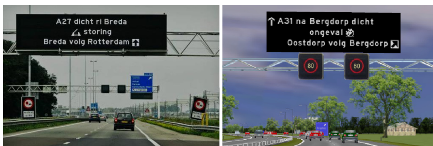
Fig. 1. Example of an overhead VMS in real-life (left) and in the driving simulator (right), informing drivers they have to deviate from their route. Translations of the VMS texts are “A27 to Breda is closed. [Bridge] Malfunction. Breda follow Rotterdam” (left) and “A31 closed after Bergdorp. Accident. Oostdorp follow Bergdorp” (right).
