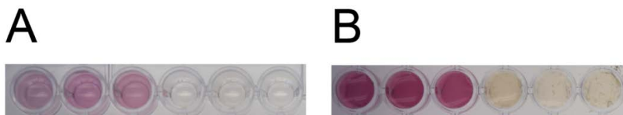
Figure 7: Test of ChitO-based assay on real substrates: A) shrimps' shell treated with chitinase from Streptomyces griseus , and B) straw treated with cellulase from Aspergillus niger . Triplicates of the substrate treated with the hydrolase (left) are compared with triplicates of non-treated substrate (right). Photos were edited to improve the contrast.
