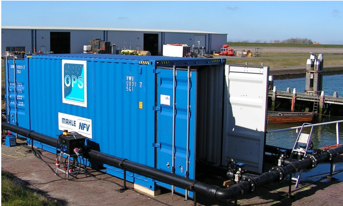
Figure 5. Example of a ballast water treatment system inside a 20 foot container, tested at the NIOZ harbour. (Photo: P. P. Stehouwer)
