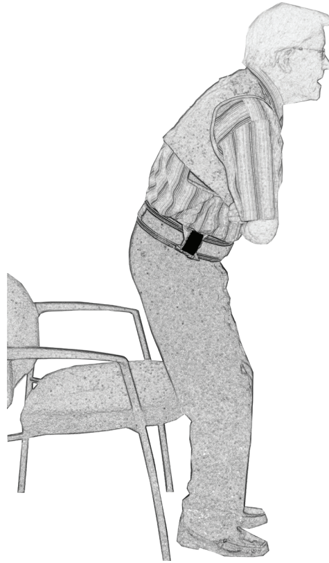
Figure 2 | A motion sensor can be used to estimate power during the sit-to-stand movement. The small black box on the right side of the hip represents a body-fixed motion sensor. The vertical acceleration signal measured with the motion sensor can be used to estimate the vertical peak power of the body's center of mass during the sit-to-stand transfer [38].
