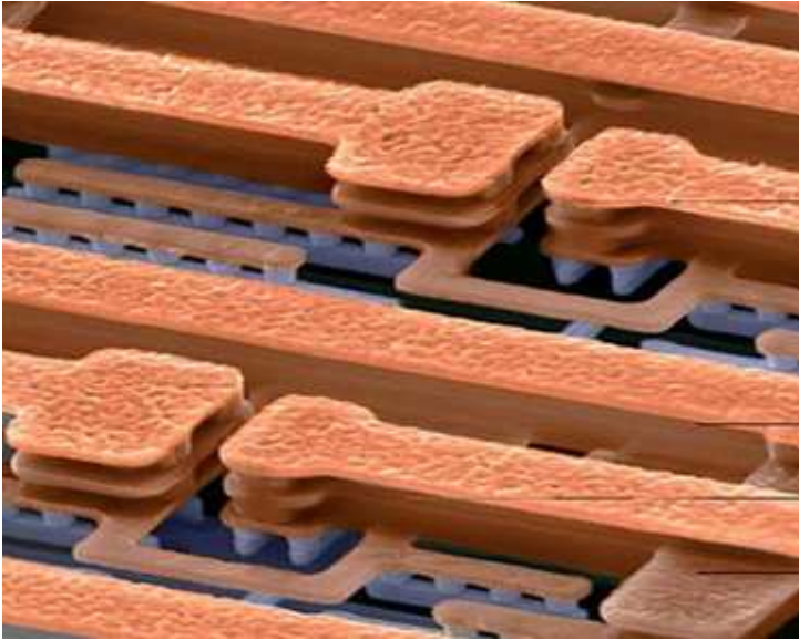
Figure 3.1: Metal interconnects in an integrated circuit device [1]. Image courtesy of IBM.
