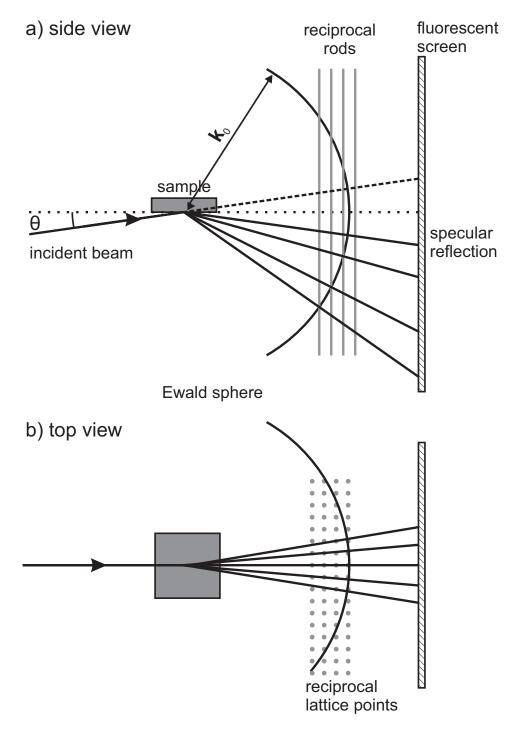
**Figure 2.4:** Ewald's sphere construction and diffraction geometry of RHEED. a) side view. The intersections of the Ewald's sphere with the reciprocal space rods are the positions where the diffraction conditions are fulfilled. b) Top view.
