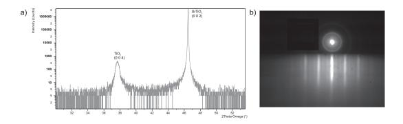
**Figure 2.10:** a) XRD pattern showing the  $TiO_2$  (anatase) (004) reflection and the (002) Sr $TiO_3$  substrate peak. b) RHEED pattern of a  $TiO_2$  thin film, showing satellite peaks close to the main spots that are typical for anatase [62]
