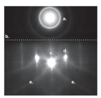
**Figure 2.5:** RHEED pattern of a SrTiO<sub>3</sub> substrate. a) direct beam. b) shadow edge, c) specular (00) spot. d) off-specular (01) spot. e) Kikuchi lines
