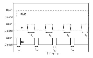
**Figure 2.11**: Shuttering scheme used for  $Pb_xSr_{1-x}TiO_3$  growth. The titanium time corresponds to a single monolayer. The Strontium time determines the level of substitution.
