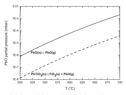
**Figure 2.12:** Phase diagram of PbTiO<sub>3</sub> as a function on PbO partial pressure and temperature. After Theis et al. [87]
