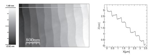
**Figure 2.7:** Tapping mode AFM image of a treated SrTiO<sub>3</sub> substrate. The profile clearly shows a step size of  $\approx$  3.9 Å
