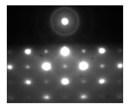
Figure 2.6: 3D transmission pattern of PbO islands on SrTiO<sub>3</sub>
