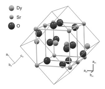
**Figure 2.8**: Structure of DyScO<sub>3</sub>. The edges of both the orthorhombic and pseudo-cubic unit cell are shown.
