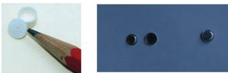
Figure 2.9: Left: alumina crucible with a lid used for high temperature DSC-TGA. Right: open and closed pans used for low temperature DSC.
