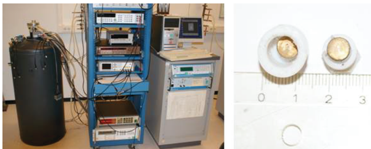
Figure 2.8: Picture of Quantum Design PPMS and specially made Teflon parallel plate sample holder for capacitance measurements.
