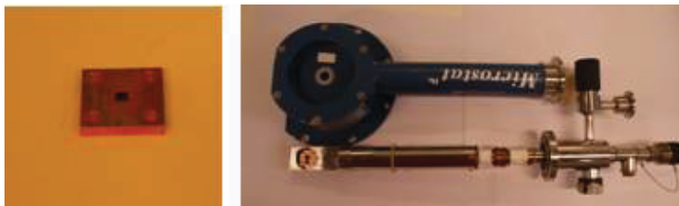
Fig 2.10: Copper sample holder and Oxford cold finger used for temperature and pressure (vacuum) dependent Raman spectroscopy.
