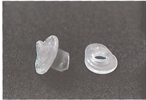
Fig. 1. Deposits on the esophageal flange and valve-seating of a dysfunctional Provox™ voice prosthesis.
