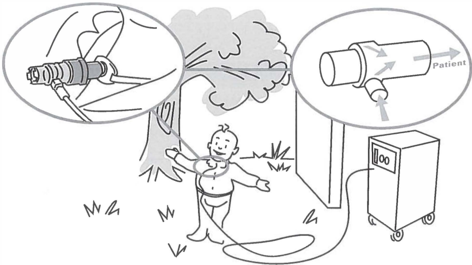
Figure 6.1 Schematic diagram showing the delivery of continuous positive airway pressure (CPAP) to an infant at home.
