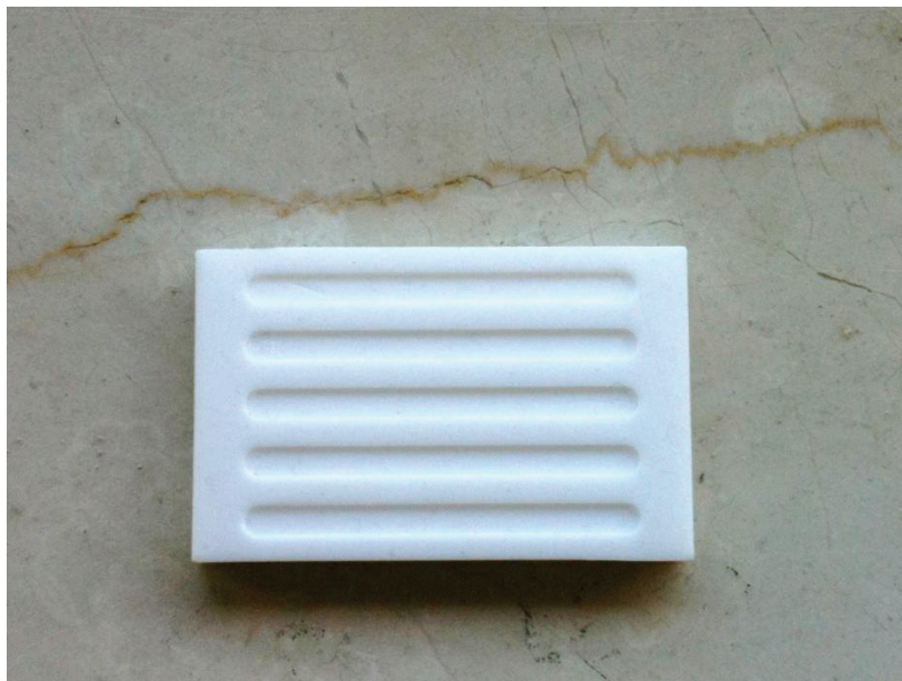
Figure 4.1. The teflon mold for preparing polyurethane networks. The dimension of the strip space of mold was 40x3.0x0.8mm.
