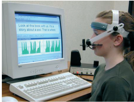
Figure 6: Kay Pentax nasometer II software installed on a computer, hardware on the table and headgear installed on a subject. 30
