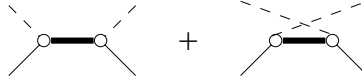
Figure 2.1: The sum of diagrams included in the calculation of the K matrix in the model with nucleons and pions only. The solid lines are nucleons, the dashed lines pions. The nucleon propagators are dressed, as indicated by the thicker lines. The circle represents the dressed \pi NN vertex.
