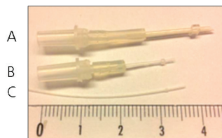
Figure 4. Cannulas. Cannulas for the portal vein (A) , celiac trunk (hepatic artery) (B) and common bile duct (C) . Cannulas are composed of pieces of tubing slid over one another, with a small ring of tubing at the tip to prevent them from being pulled out of the blood vessel or bile duct.
