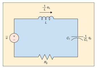
Figure 1. Series RLC circuit.
