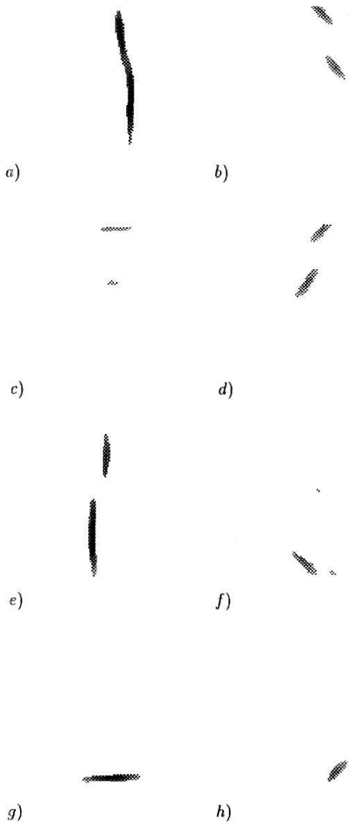
Figure 3: Cortical images computed from the input image shown in Fig.2a using antisymmetric receptive field functions of different orientations: a) \Theta = 0, \varphi = -\frac{1}{2}\pi , b) \Theta = \frac{1}{4}\pi, \varphi = -\frac{1}{2}\pi , c) \Theta = \frac{2}{4}\pi, \varphi = -\frac{1}{2}\pi , d) \Theta = \frac{3}{4}\pi, \varphi = -\frac{1}{2}\pi , e) \Theta = 0, \varphi = \frac{1}{2}\pi , f) \Theta = \frac{1}{4}\pi, \varphi = \frac{1}{2}\pi , g) \Theta = \frac{2}{4}\pi, \varphi = \frac{1}{2}\pi , h) \Theta = \frac{3}{4}\pi, \varphi = \frac{1}{2}\pi . The values of the other receptive field function parameters are: \sigma = 32, \gamma = 0.5, \lambda = 2\sigma . (Image size 512 \times 512 .)
