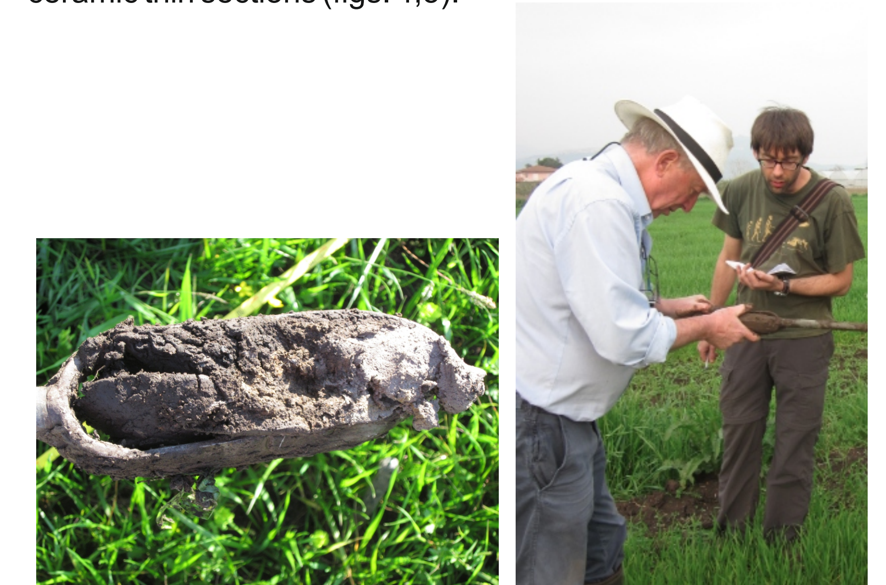
Figure 4: Collection of a clay sample using an auger.
