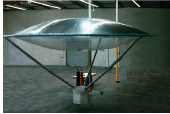
FIG. 1.1. An inflatable space reflector test setup of the company L'garde ( www.lgarde.com ).
