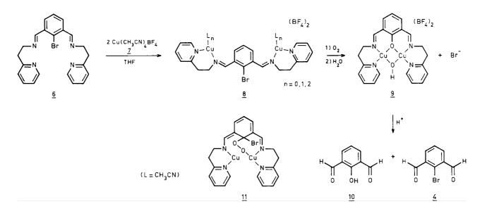
observed. Isolation and characterization of the oxidation product after 16 h. showed that dinuclear Cu(II) complex <u>9</u> had been formed in about 80% yield. Hydrolysis of the reaction mixture, using aqueous HCl, gave the corresponding phenol (yield 80%) together with unreacted bromodialdehyde <u>4</u>
