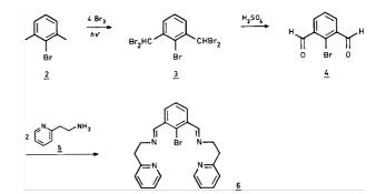
The tetradentate ligand <u>6</u> reacts with two equivalents of  $Cu(CH_3CN)_4BF_4(7)$  in dry THF under an inert nitrogen atmosphere to produce, after it was washed several times with THF, a pure orange binuclear Cu(I) complex [Cu<sub>2</sub>(2,6-BPB-1-Br)(BF<sub>4</sub>)<sub>2</sub> 1.8 CH<sub>3</sub>CN].(<u>8</u>)
