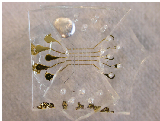
Figure 1.14: Picture of an home made PDMS-Au TS -SAM//EGaIn-PDMS device.
