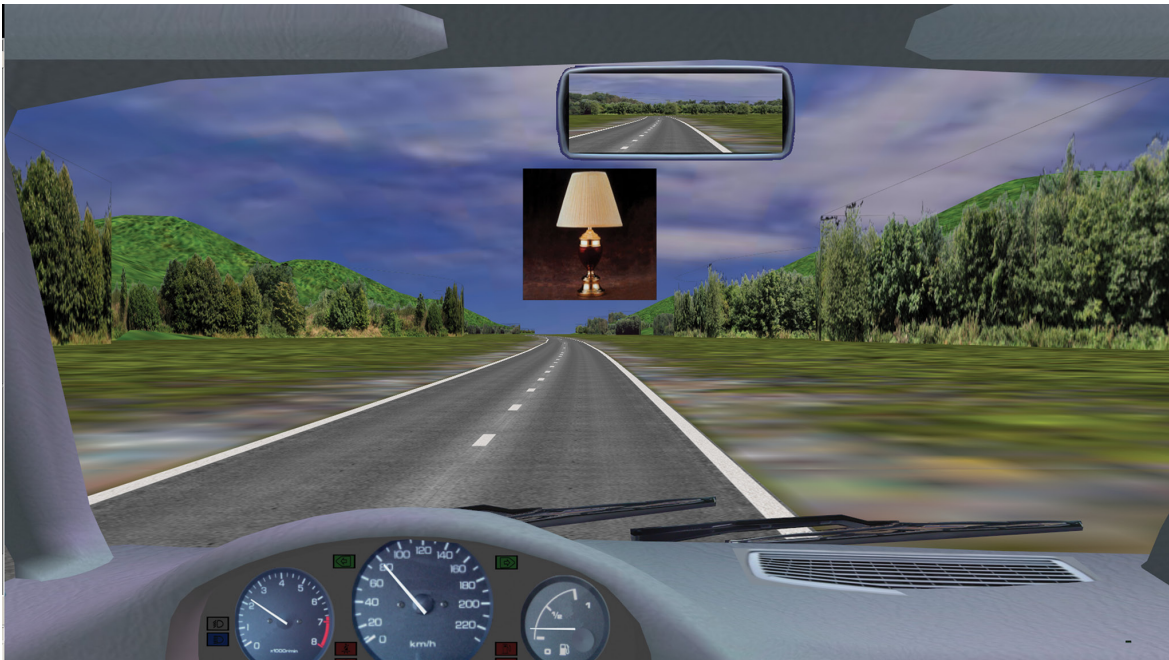
Figure 6.2. Screenshot of the simulator's centre screen showing the road environment and an example masking image in the position in which the images were presented during the trials.
