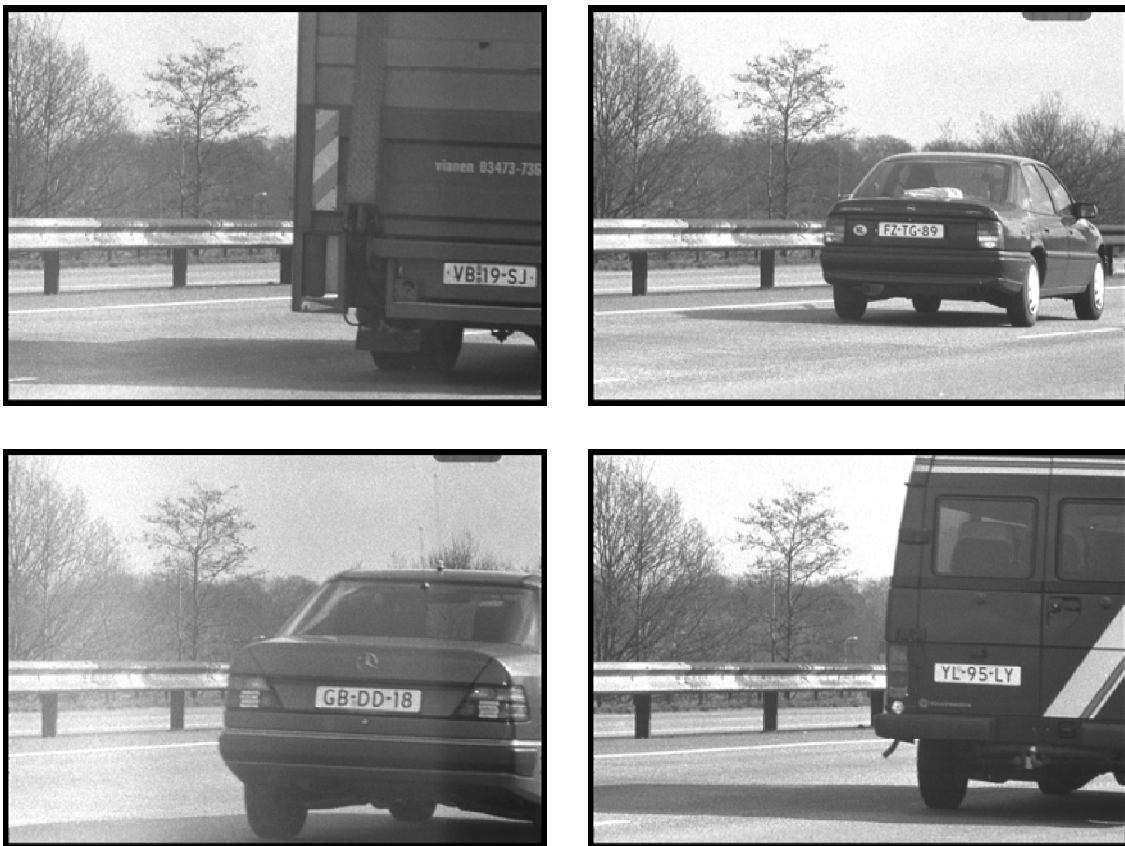
Figure 7.1: Some input examples for the CLPR system. The images are recorded by a police-operated monitoring system. Each image contains 768 \times 567 pixels with 8-bit gray scale information per pixel.
