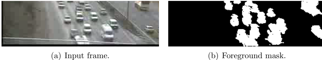
Figure 3.6: Results of the enhanced adaptive background mixture model.
