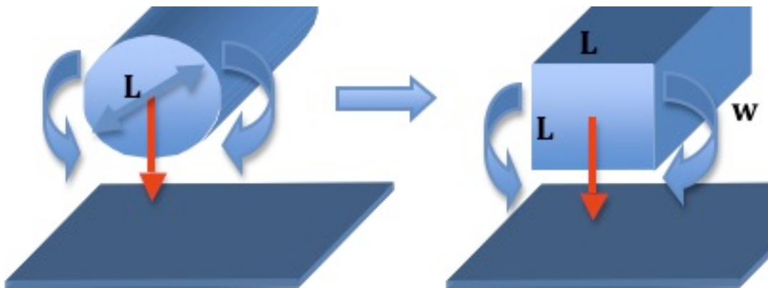
Figure 13: Schematic demonstrating similarity between cylindrical body and square beam approaching deformable surface, with the lubrication forces depicted as equivalent moments.
