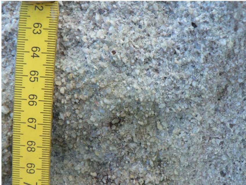
Figure 2.11: Very coarse grained sand at Chalky Mount Ridge. Tape measure is in cm.
