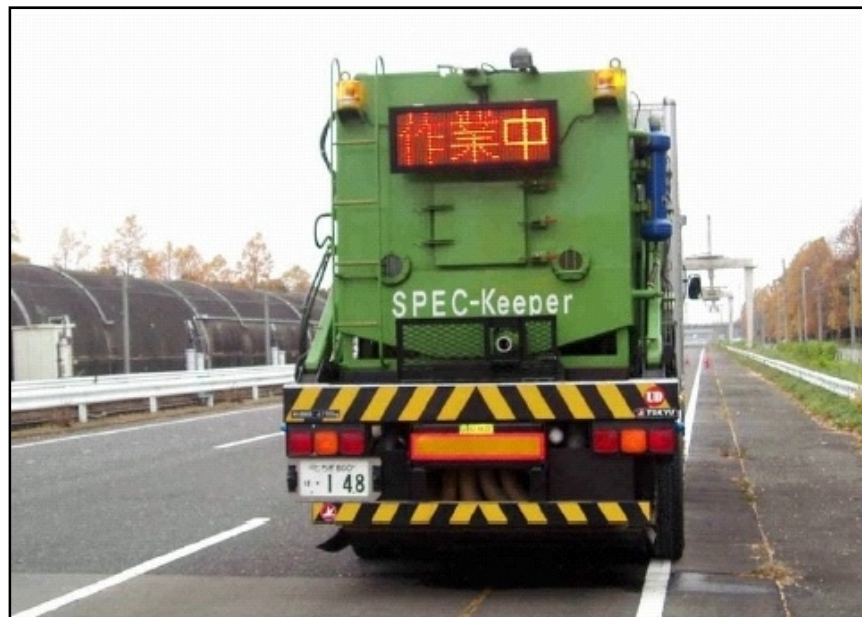
Figure 13 - The Spec-Keeper cleaning machine in Japan from PWRI (2005)
