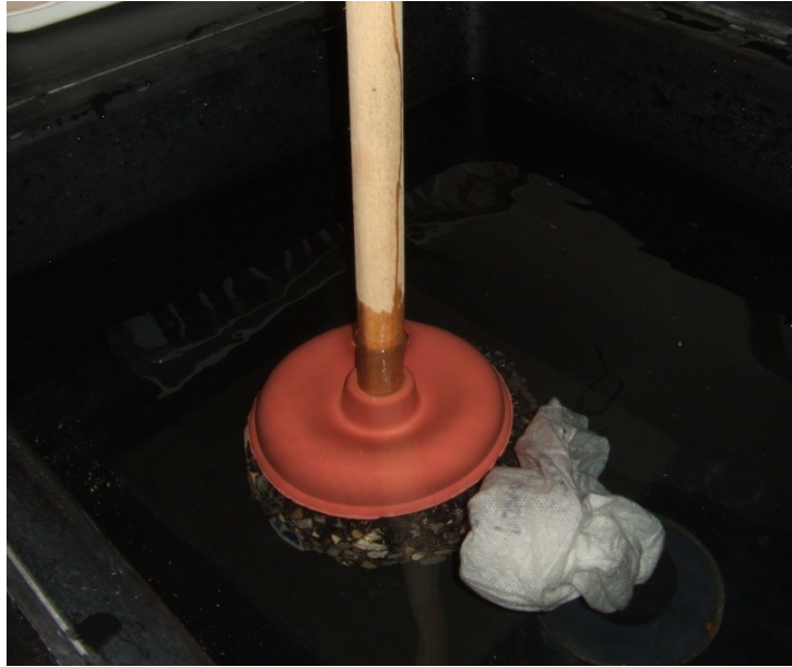
Figure 26 - Plunger unclogging a PFC core
