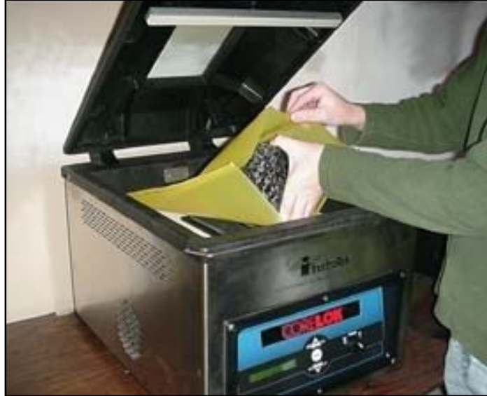
Figure 15 - Enclosing the Sample in the Plastic Bag – CoreLok device
