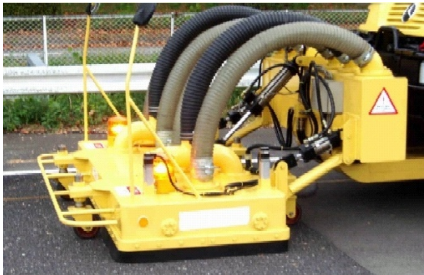
Figure 14 - Cleaning Machine with High Pressure Air only from PWRI (2005)
