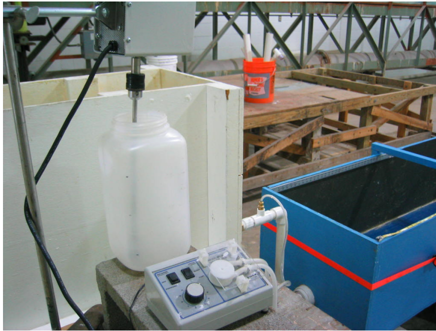
Figure 4.9. Particle delivery system for the second trial
