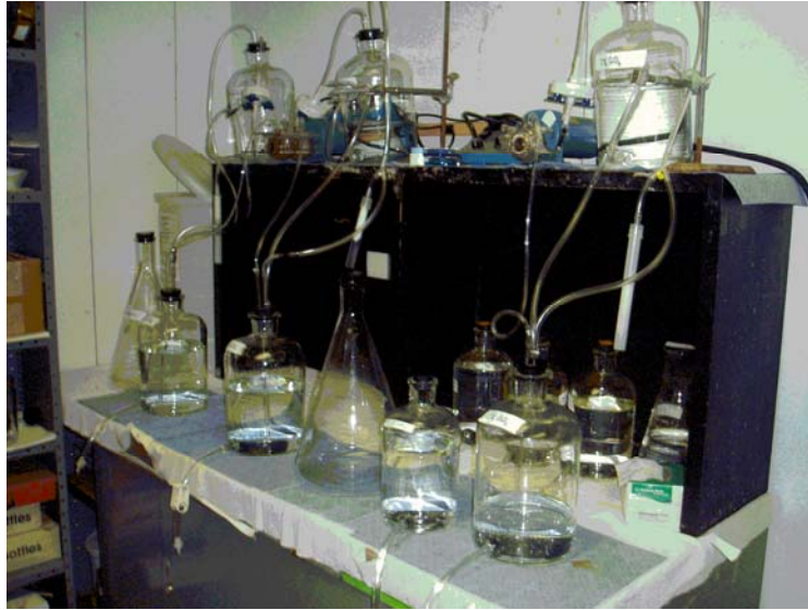
Figure 3.5 Electrolyte Filtering Set-up
