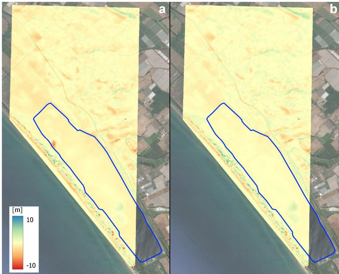
**Figure 3:** The difference in height between the 1928 DEM and the LIDAR DTM; a) without the height shift, b) with the height shift. The blue line is the contour of the modern Caprolace lake.
