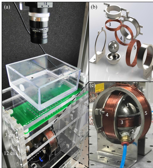
Fig. 5. The spherical electromagnetic actuator consists of coils, actuator magnet, sensor board, and a reservoir. (a) A 5 mm roller moves in a workspace of 5 \times 5 cm on a flat surface. (b) and (c) The field is generated using a permanent magnet (1), and an air-bearing (2) reduces its friction. Coils (3), (4) and (5) control the orientation of the permanent magnet.
