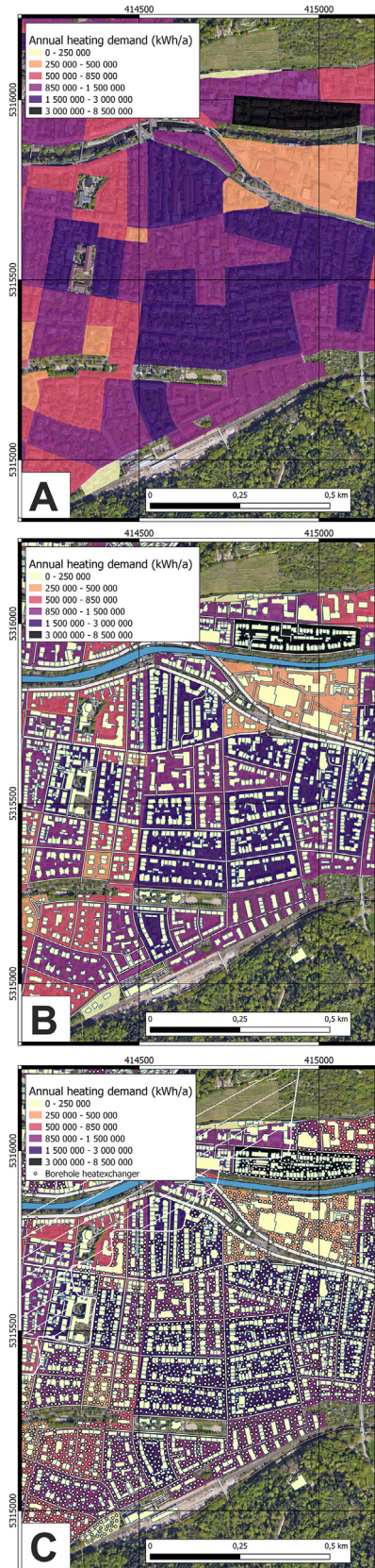
Fig. 3. Maps illustrating the process of distributing BHEs: (A) shows the annual heating demand per building block. (B) For each building block unsuitable areas (buildings, roads, railways, waterways) are excluded. (C) BHEs are randomly distributed with a 10 m spacing to maximise the amount of BHEs available per building block.
