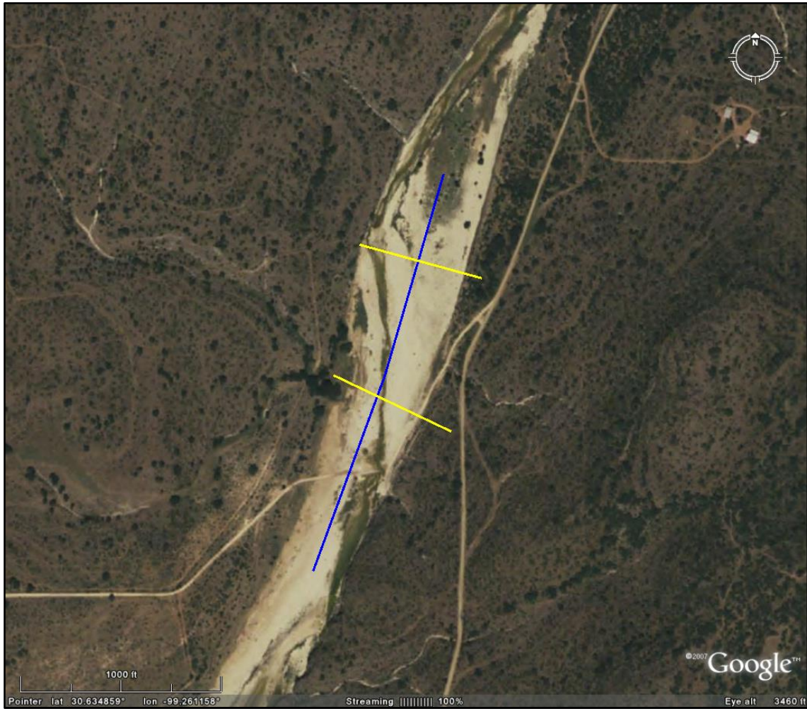
Figure 4.2. Two cross-section transects (yellow lines) and flow path (blue line) of the James River near Mason, Texas. For scale, yellow lines approximately are 250 meters. Flow direction is toward the north-northeast (upper part of the image). Natural-color imagery from Google Earth, accessed in February 2008.
