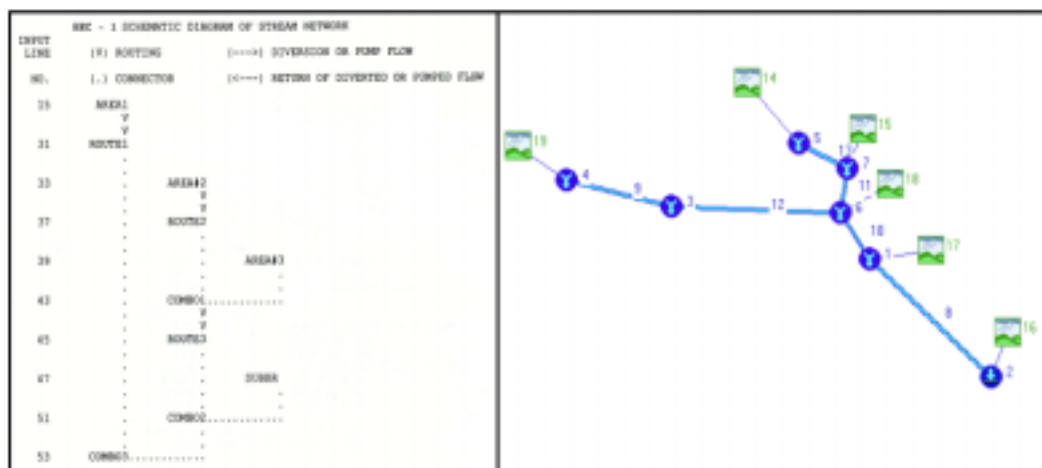
Figure 6-1 Comparison of HEC-1 and HEC-HMS Stream Network Schematic Diagrams without SCS Flood Control Structures
